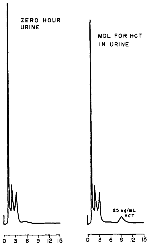
Figure 8. HPLC Chromatograms of extracts of a zero-hour equine urine (left) and a zero hour equine urine spiked with 25 ng/ml hydrochlorothiazide (right) This level of HCT in urine represents the practical minimum detectable limit.
